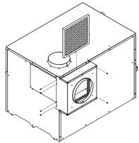
FIG. 24 Attaching DV Box Adapter to Unit
